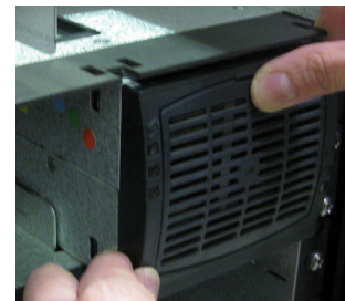
Figure 48 — Unlocking and locking an inverter module for removal or insertion
