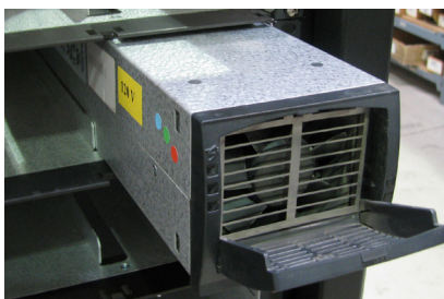
Figure 48 — Unlocking and locking an inverter module for removal or insertion
