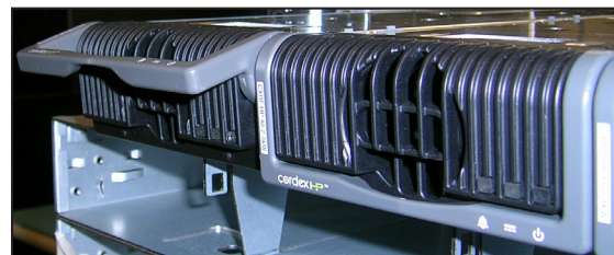
Figure 44 — Locking handle disengaged/engaged
