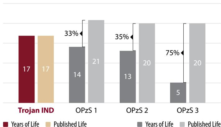
The graph above shows the equivalent years of life versus the published life. Trojan Industrial Line testing resulted in the same 17 years of life as Trojan reports in its product data.
