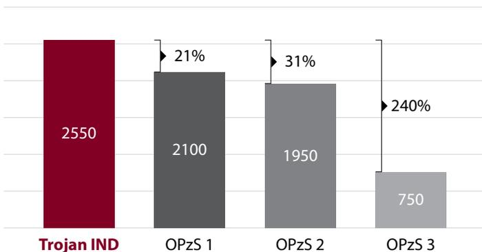
The graph above shows that the Trojan Industrial Line outperformed the three OPzS batteries tested, and depicts 21% more cycles than the OPzS 1, 31% more cycles than the OPzS 2, and 240% than the OPzS 3.
