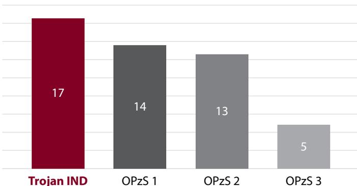
The graph above shows the equivalent years of life. Every 150 cycles under the IEC 61427 test is equal to 1 year of life in the field. The Trojan Industrial Line testing shows it to last 17 years versus the OPzS 1 of 14 years, OPzS 2 of 13 years and OPzS 3 of 5 years.
